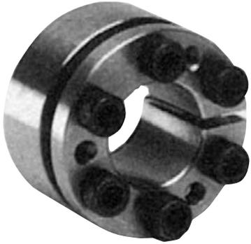
These shaft clamping elements are very compact units capable of transmitting medium torques. Their design ensures good concentricity between hubs and shafts, without any other means of location. A slight axial movement between hub and shaft occurs during clamping. These units can be installed totally within the hub providing optimum safety, and minimal axial length.
