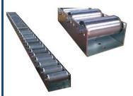
Available rollers are Ø40, Ø50 or Ø60 set at 52, 78 or 104mm pitch. Rollers are bolted in position to make for secure fixing but can be easily removed to allow additional rollers/brake rollers to be fitted.
