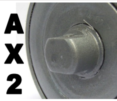
AX2 M/CD FLATS Top and bottom of axle are flattened
